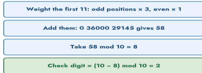
Figure 5. The UPC-A check digit makes the full weighted sum reach 0 modulo 10.
